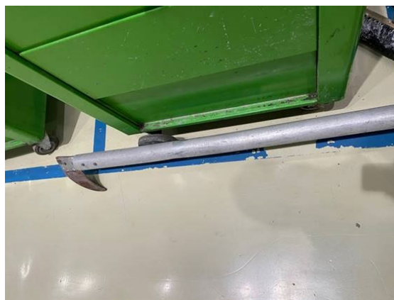
Hook to remove broke (SCP example)
