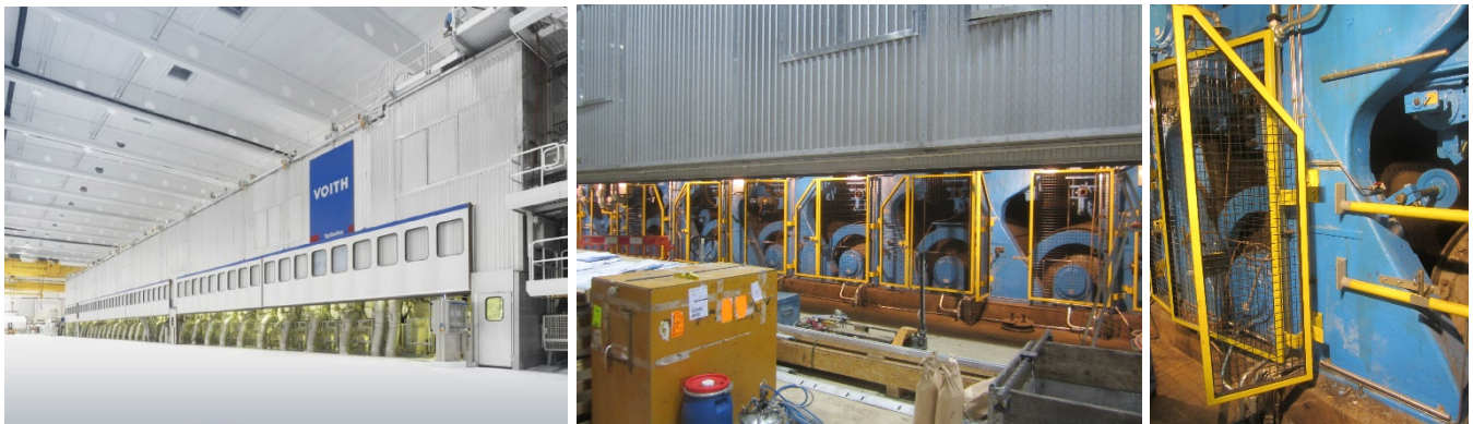
Examples of drying section paper machine guarding
